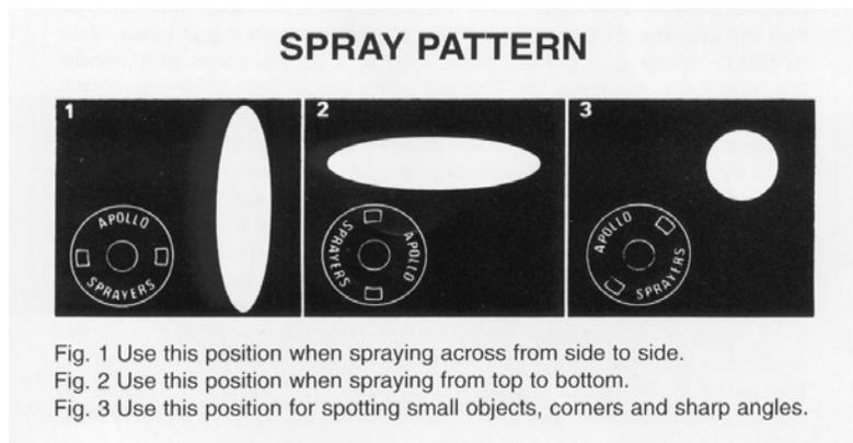
Fig. 1 Use this position when spraying across from side to side.
